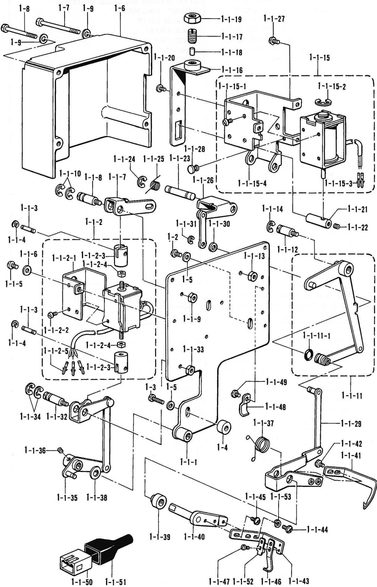
N. 糸ツカミ関係/Thread clamp mechanism/Nahtanfänge/
