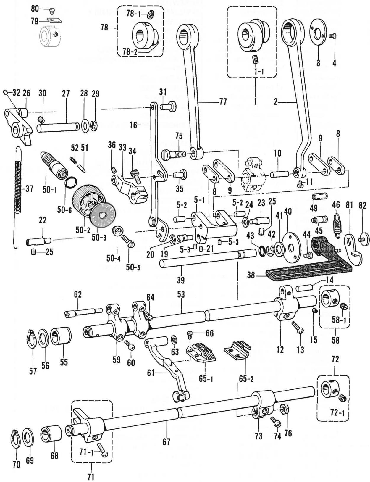
E. 送り関係/Feed mechanism/Transportvorrichtung/
