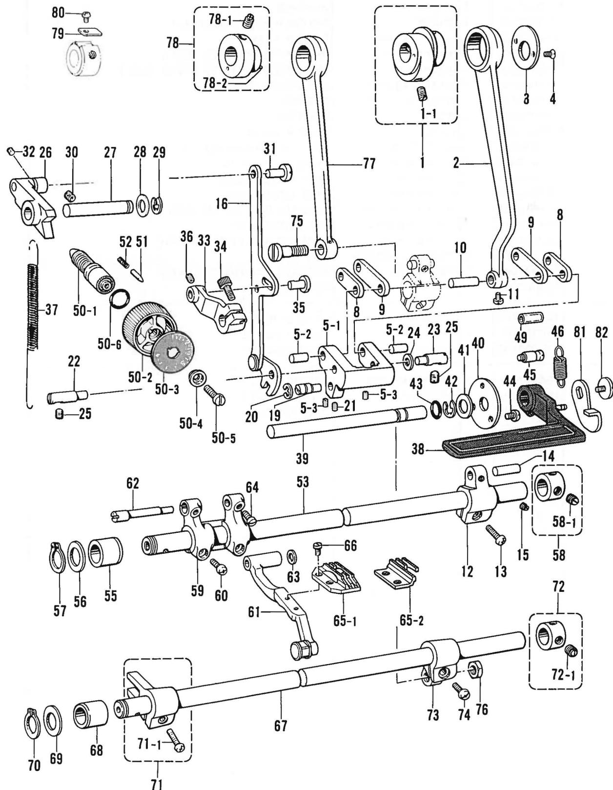
E. 送り関係 / Feed mechanism / Transportvorrichtung /
